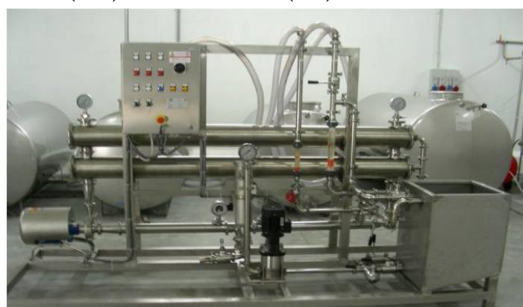
Figure 1. Separation system based on membrane technology: Microfiltration (MF), Ultrafiltration (UF) and Reverse Osmosis (RO).
